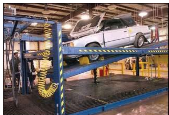
Fluids and heavy metals are removed in a building on the lot. This car is being tilted to make the process easier. For vehicles, U-Pull-&Pay is the last stop before the crusher.
